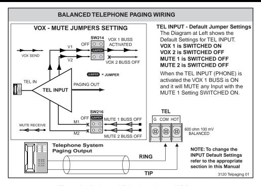
Fig. 13A - Balanced Telephone Input Wiring
